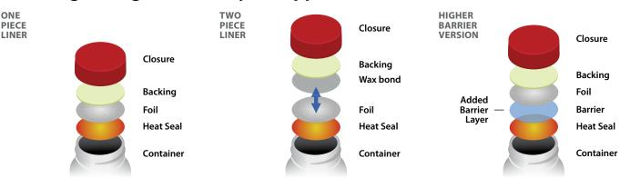
Induction seals prevent leaks and preserve product freshness. Packagers should specify whether the induction liner will peel away cleanly or leave indication of tamper evidence. Peelable liners can include tabs which make the liner easier to remove.
